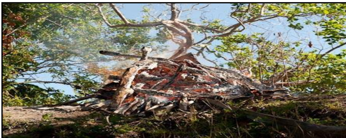
The dried coral being burnt using dry hard wood
