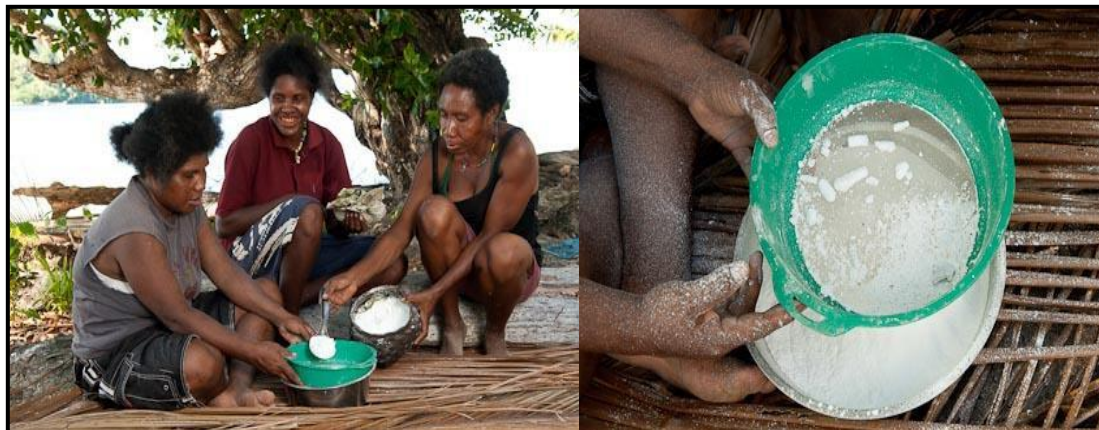
After sieving the residue of burnt coral are separated from the powder
